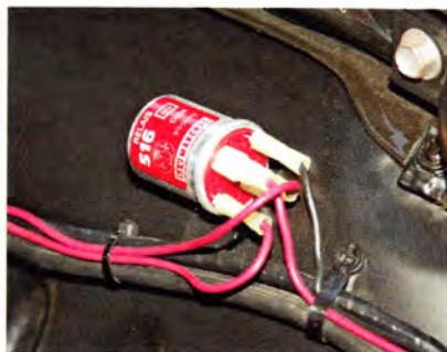
The Marchal foglamps were activated by this relay mounted on the inner fenderwell.
